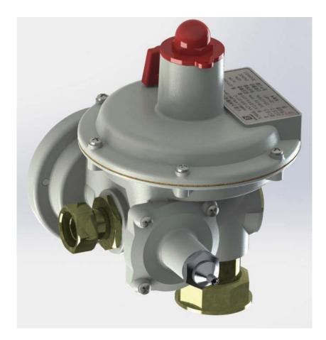
Construction and performance features make the LQ 50/70 /100series spring-loaded regulators the ideal choice in applications involving sudden changes in capacity or where the gas shut-off is solenoid-controlled as with domestic or industrial burners. These regulators can be employed with natural, manufactured, propane, air and other gases so long as they are duly filtered and do not contain high percentages of benzol.
